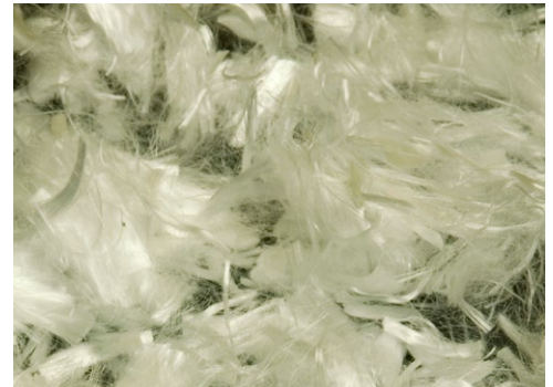
FiberMaxMI fibers help prevent micro cracks that form as water evaporates from concrete.
